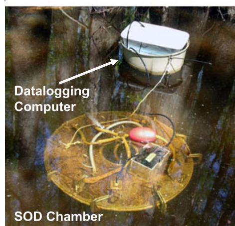
FIGURE 3. (a) Schematic of Sediment Oxygen Demand Chamber and (b) Typical Deployment of Sediment Oxygen Demand Chamber and Associated Data Logger in the Field.
