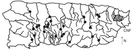
Figure 1. Map of Puerto Rico showing major stream drainages, locations of completed large dams (height >15m, black dots), an additional large dam under construction on the Río Portugués (open dot), and the Caribbean National Forest (CNF).
